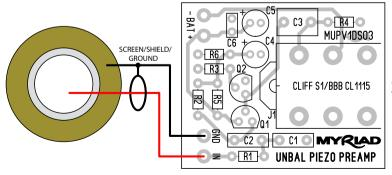
1/4" Mono Jack Output Tip - signal Sleeve - GND
